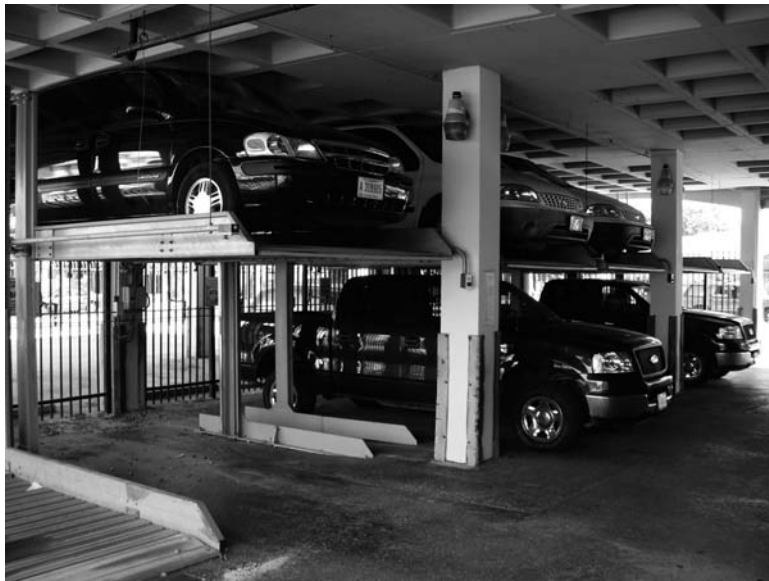
Figure 8.4 Dual-Layer Stacked Car-Parking System, Miami, Florida
