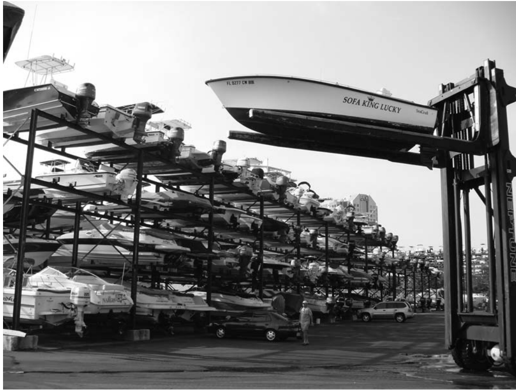
Figure 8.5 Quad-Layer Stacked Boat-Parking System
